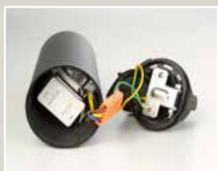
CCT and power switches within body
